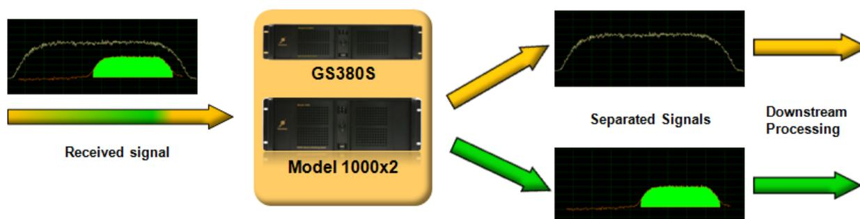
**GS380S Separates Signals for Downstream Processing**
