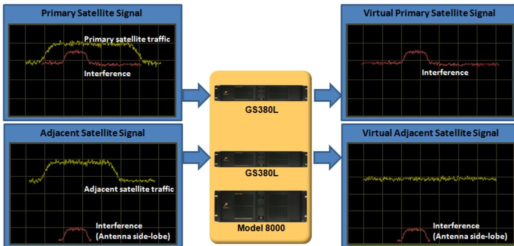
**GS380L Removes Obstructing Signals to Enhance Geolocation Performance**
