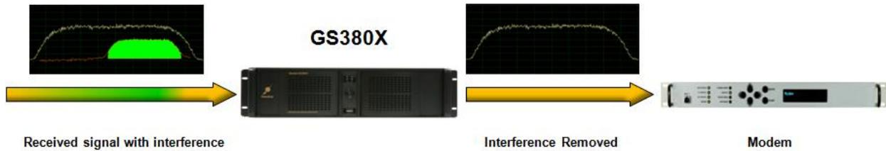
**GS380X Streaming Interference Removal Improves Receive Performance**
